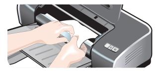
After you clear the jam, close all covers, turn on the printer (if you turned it off), and press the Resume button. The printer will continue the print job on the next page. You will need to resend any pages that were jammed in the printer.
